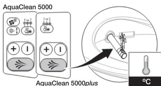
**i** If the storage or transport temperature exceeds 45 °C, the safety thermostat will be tripped.
